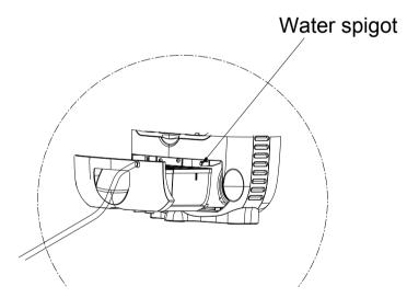
If you find that the water does not flow down the hose then check that it is running downhill, is not kinked, all excess tube has been cut off and is not blocked. If the water still does not flow then make a 4mm hole, 30mm from the spout in the top of the hose. This will balance out the air pressure and allow the water to flow.
